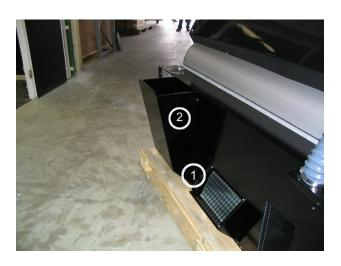
⇒Put the top art of the exhaust air stack onto the fixed bottom part of the exhaust air stack ⇒ Fix the to part (2) with 3 screws to the bottom part (1) and with 3 screws to the rear of the top plate of the
